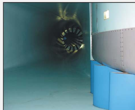
The fan blows the air into a circular room. Fins located around the bottom of the tunnel (lower right) then catch the air and push it up through the air chamber.
